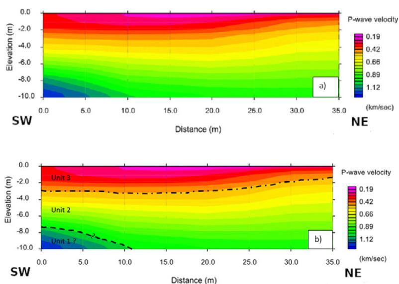
**Figure 9. The tomography results for the seismic line in the Tena River bank: a) Without interpretation. b) With seismic stratigraphic and structural interpretation.**
