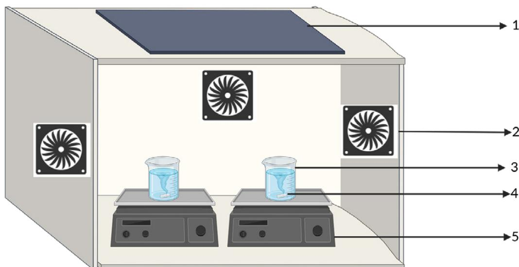
Figure 1. Schematic diagram of the experimental photoreactor for photocatalytic inactivation, which is composed of a 400W white light LED lamp (1), three fans (2), two 100 mL beakers (3), two magnetic stirring bars (4), and two magnetic stirrers (5).
