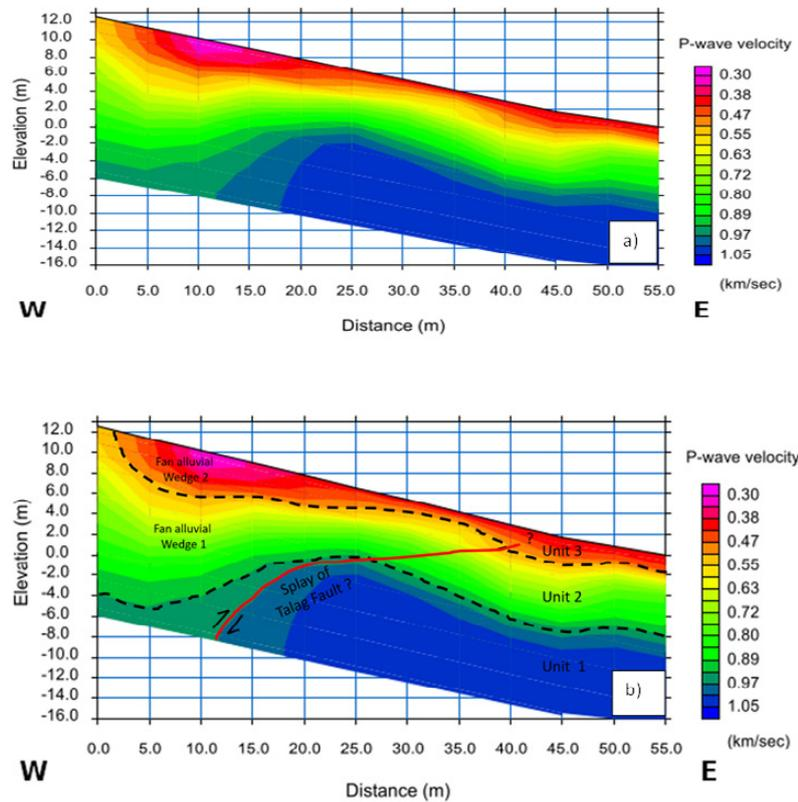
Figure 8. The tomography results for the seismic line on the Colonso-Chalupas road: a) Without interpretation. b) With seismic stratigraphic and structural interpretation.
