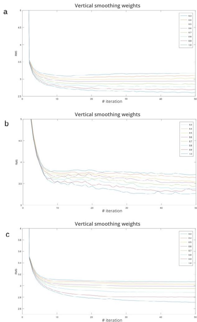
**Figure 6.** We show the tomography algorithm convergence for the three seismic lines: a) Colonso-Chalupas road, b) Tena River bank, and c) Napo River bank. In the three cases, we use 50 iterations and plot the RMS on the vertical axis. The colors give the values of the vertical smoothing parameter setting constant for the horizontal parameter: a) 1.0, b) 0.8, and c) 1.0.
