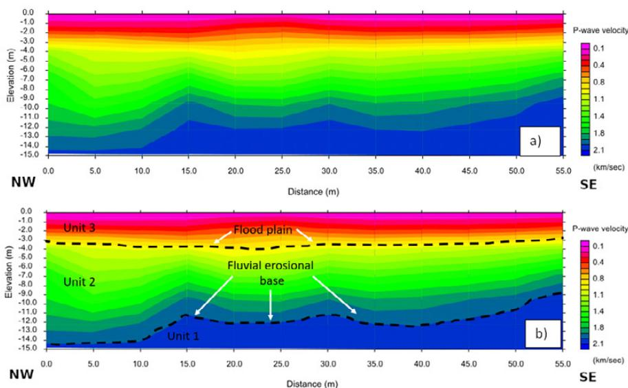
Figure 10. The tomography results for the seismic line in the Napo River bank.
